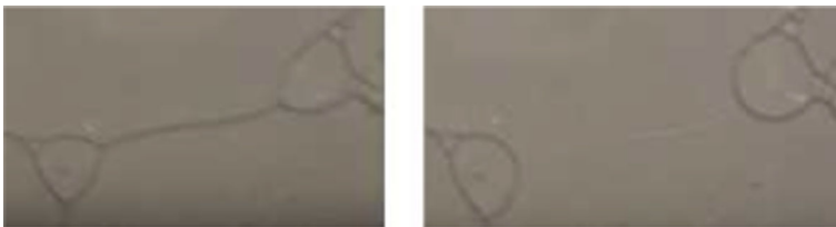
Fig. 1 An edge in a two-dimensional soap foam immediately before (left) and after (right) its rupture. The length of the edge before rupture is approximately 1 cm
